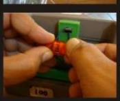
Shows twisting the flap of "TWIST SEAL" insert until it Properly locks the closure by Rotating until Most of the wire is encircled on seal insert.
